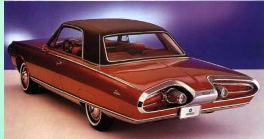
Chrysler “Turbine” (1963) – turboshaft powered consumer vehicle.
